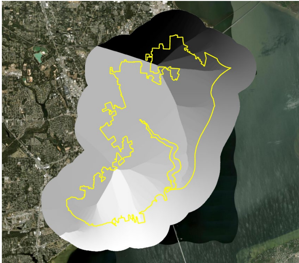
Figure 33 - Vertical Datum Interpolation Surface
