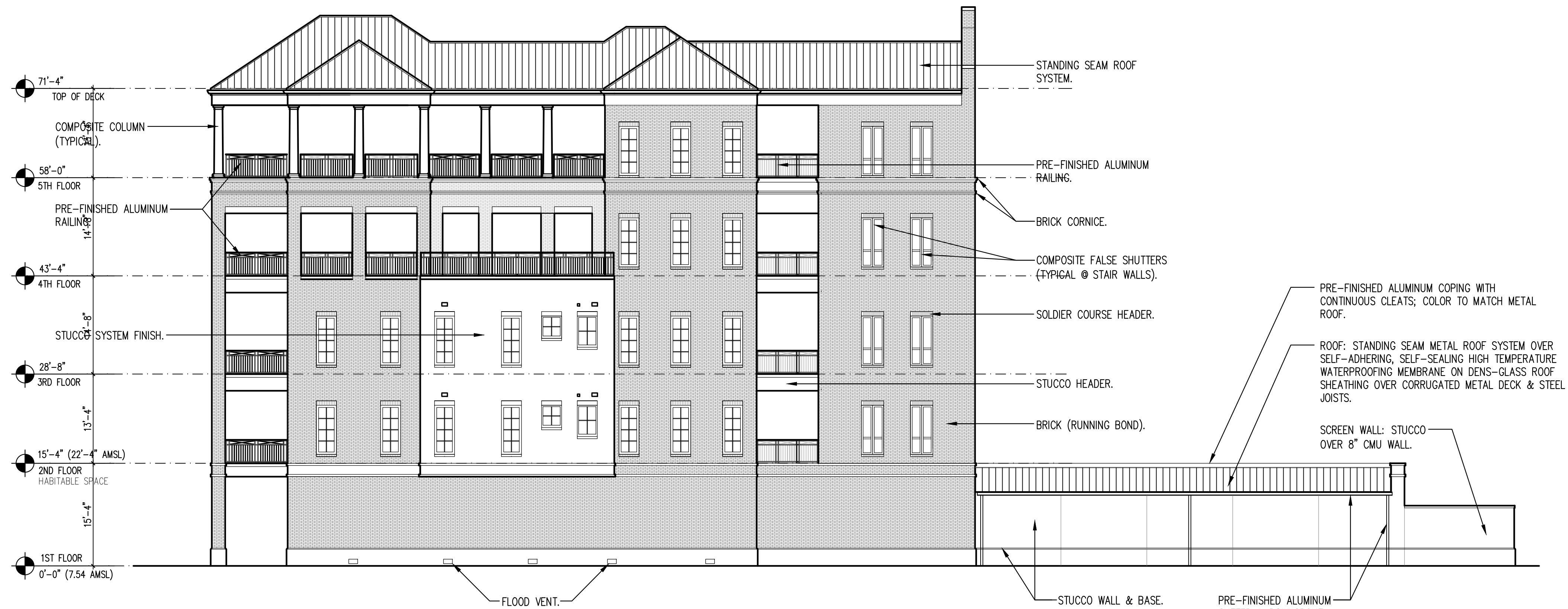
2 SOUTH ELEVATION AB-201 SCALE: 3/32" = 1'-0"
