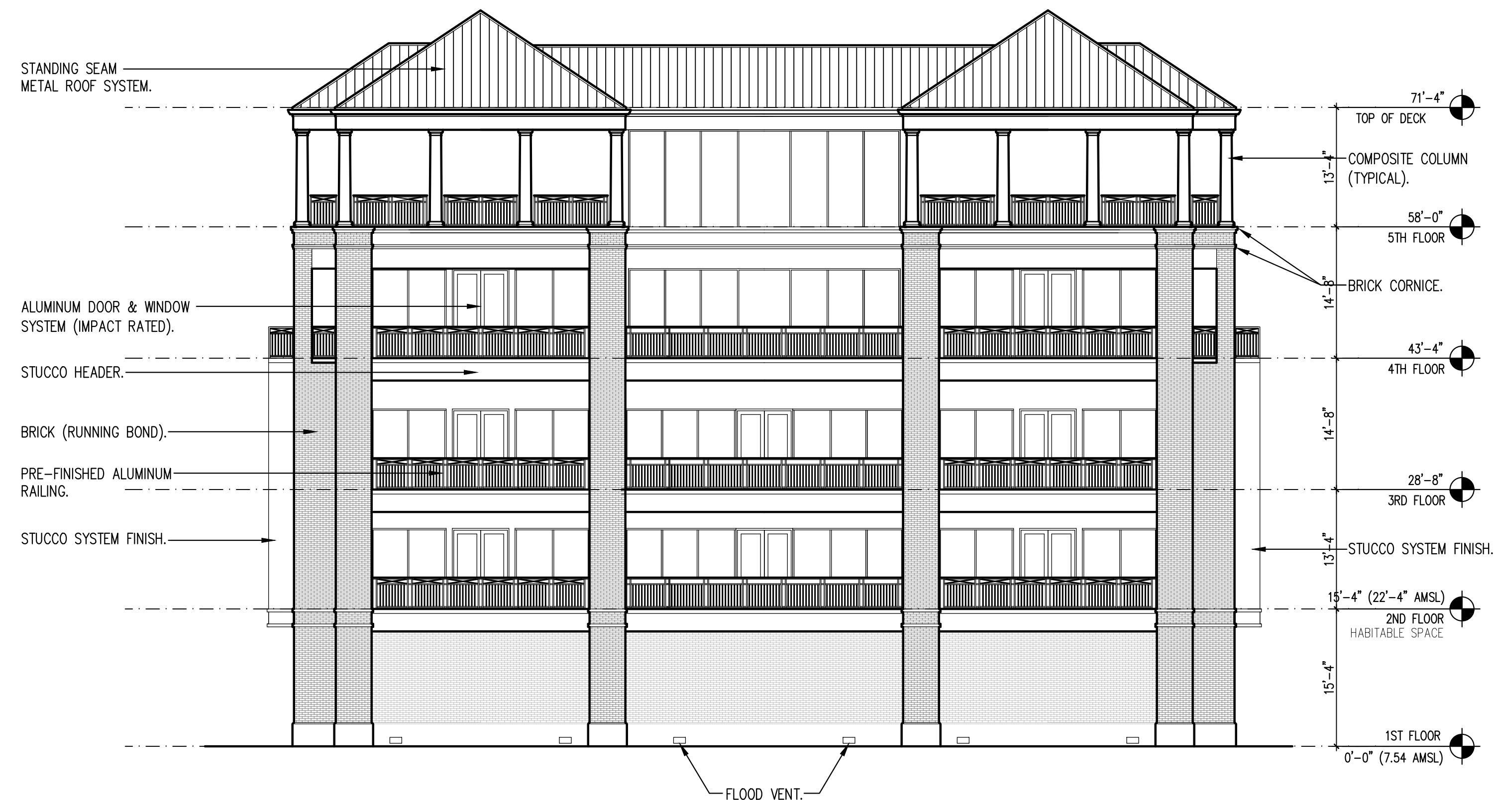
2 WEST ELEVATIONS AB-202 SCALE: 3/32" = 1'-0"
