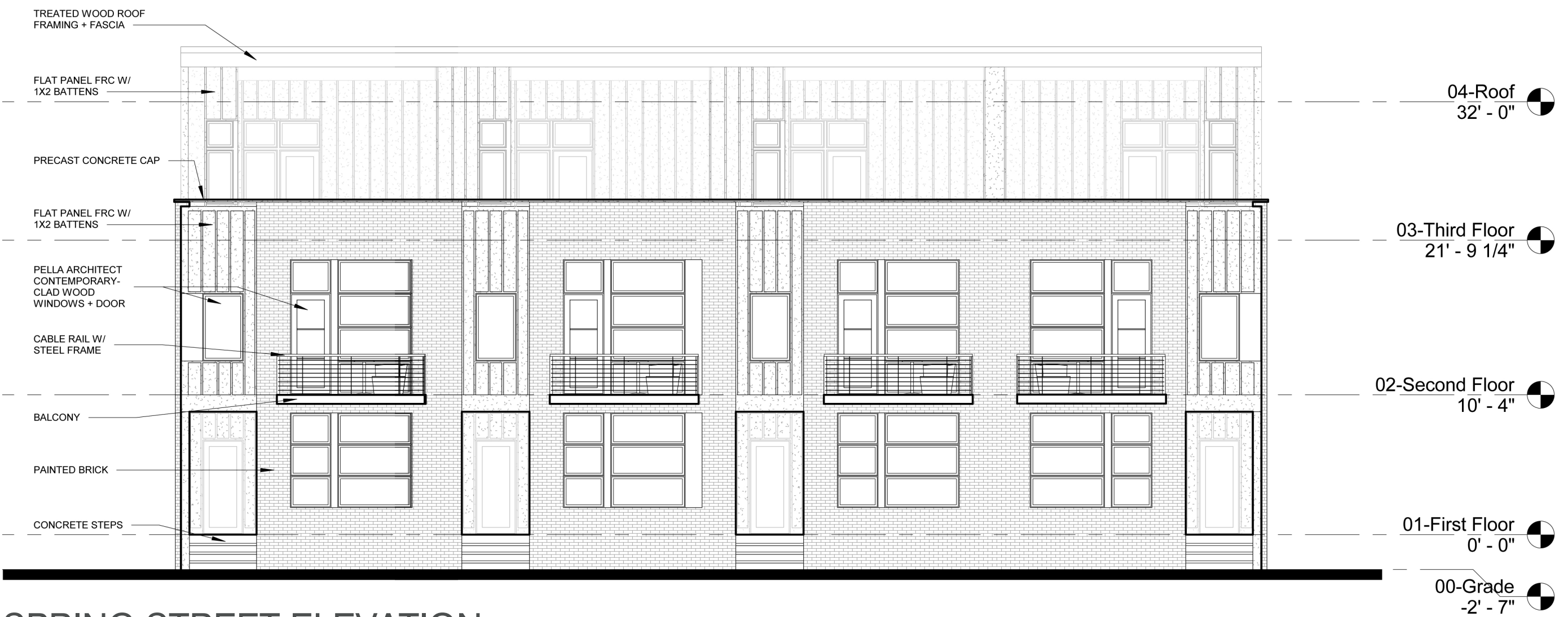
SPRING STREET ELEVATION SCALE: 1/8" = 1'-0"
