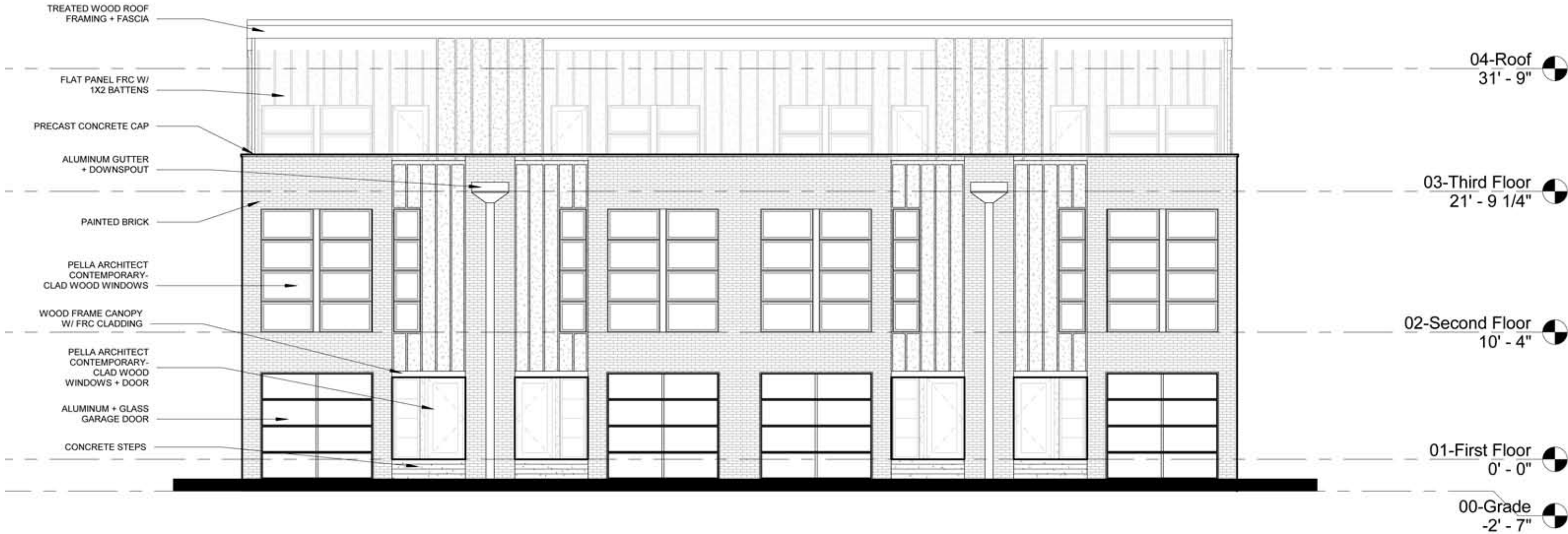
INTERIOR UNIT PARKING COURT ELEVATION (east) SCALE: 1/8" = 1'-0"
