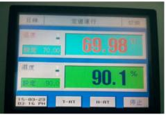
Put the whole-white cabinet into the test champer, setting it as 70°C90%RH
